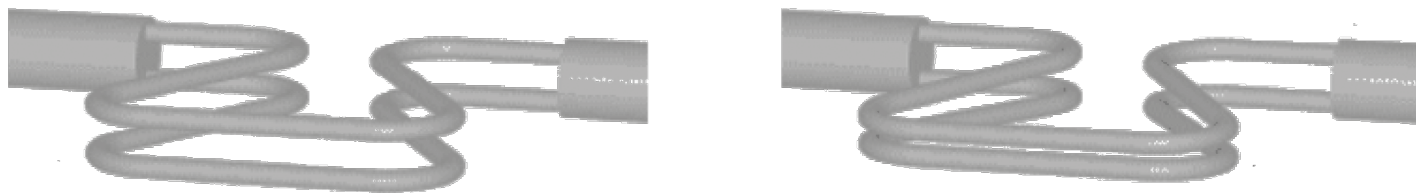
Inlet and outlet of the tubes vibrate in phase when there is no flow present.
