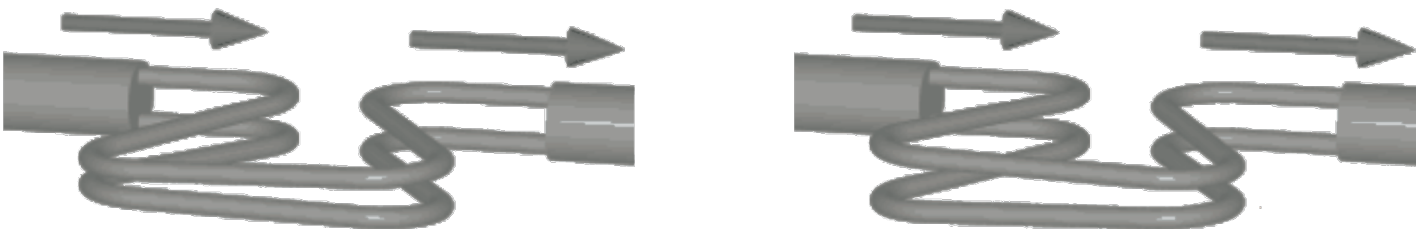
When flow is present, the inlet and outlet ends of the tube vibration is out of phase. The degree of phase shift is proportional to mass flow rate.
