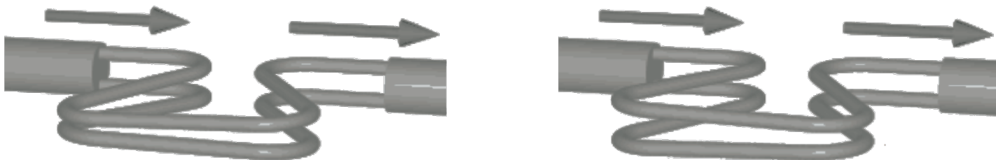
When flow is present, the inlet and outlet ends of the tube vibration is out of phase. The degree of phase shift is proportional to mass flow rate.
