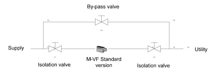
M-VF shuts the flow in the event of excess flow conditions. Close the isolation valves and attend to the problem that has caused the excess flow condition. After rectifying the problem open the isolation valves and open the by-pass valve for resetting the M-VF by equalizing pressure upstream and downstream.
