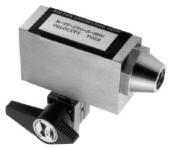
For applications where bleed to atmosphere is acceptable, such as air and nontoxic gases, the reset valve bleeds the gas behind the piston to atmosphere. This equalizes the pressure that is inside the valve and allows for a quick reset. The reset valve can then be turned off to allow the flow to resume.
