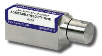
Standard version is available with positive shut off or bleed option. In the bleed option model, piston has controlled bleed, where it will reset itself after some time of shutting off the flow. The time required to reset may vary based on the operating pressure and volume of gas.
