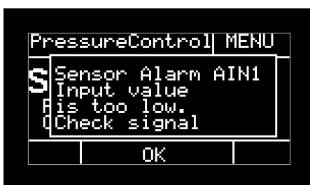
Picture 71 Sensor alarm (example)
